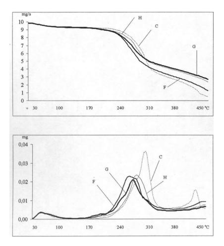
Figure 3 TG and DTG curves of the particleboards treated with Ammonium Sulfate (code F), Ammonium hydrogen Phosphate (code G) and the mixture of chemicals (code H)
