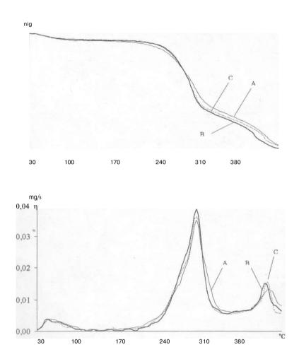
Figure 1 TG and DTG curves of the commercial (codes A and B) and the laboratory boards (code C)
