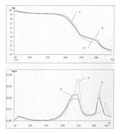
Figure 2 TG and DTG curves of the particleboards treated with waterglass (codes D and E) and the untreated (code C)
